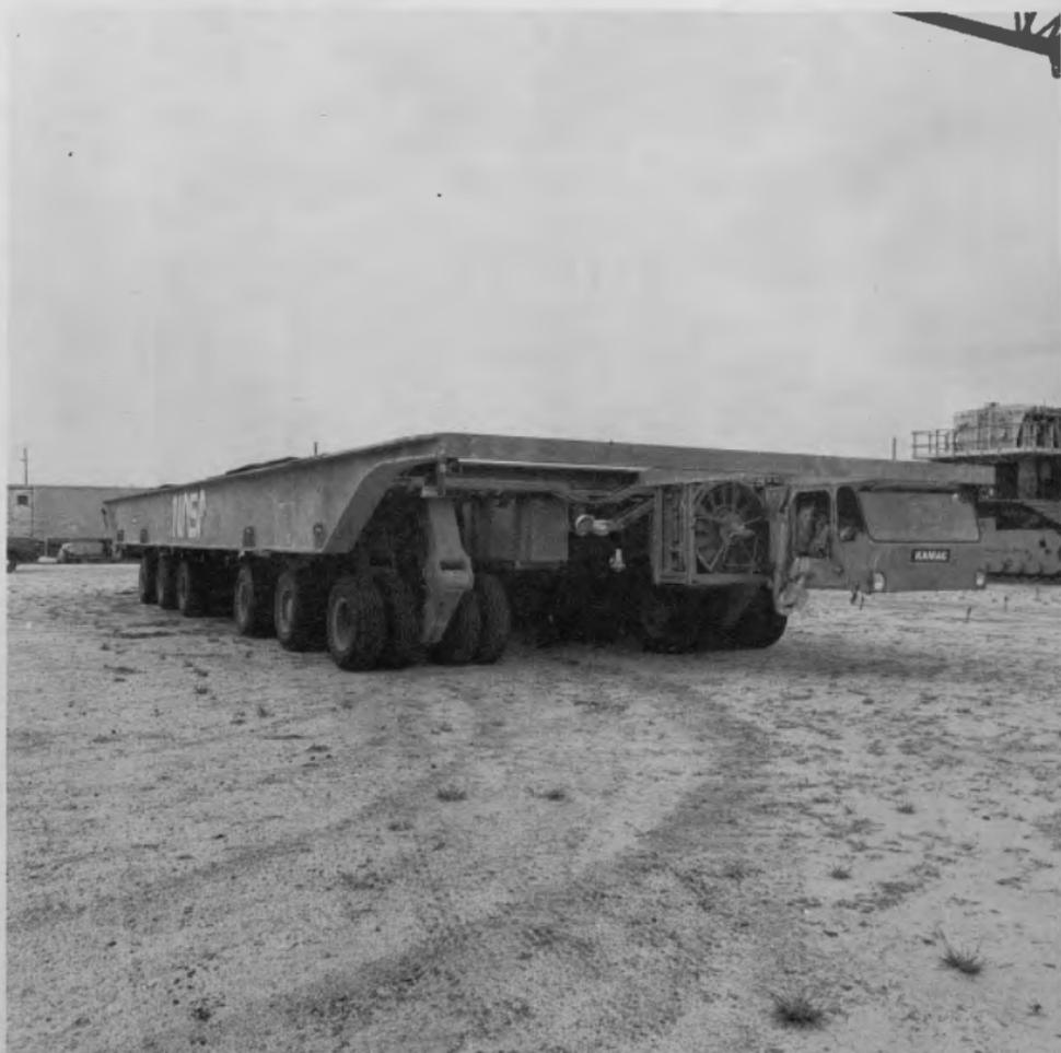
Figure 16. Payload Canister Transporter.
